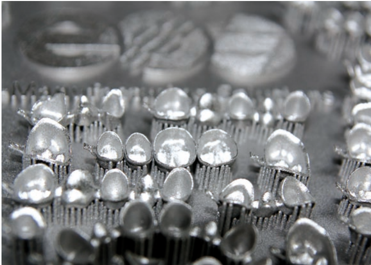
Dental platform with copings laser-sintered on EOSINT M 270.
