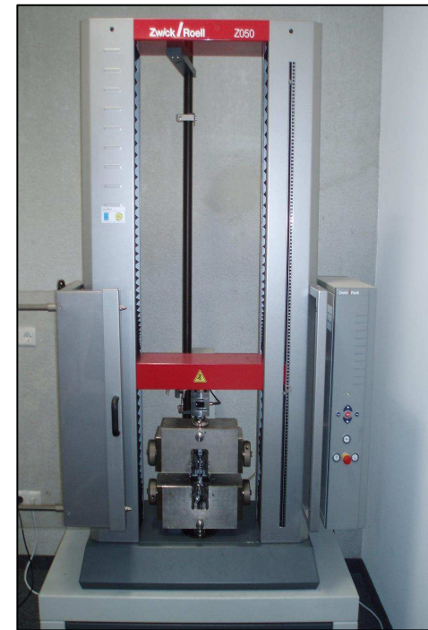
Zwick / Roell Z050, max. force 50kN, force accuracy according to ISO 7500-1, extensometer accuracy according to ISO 9513
